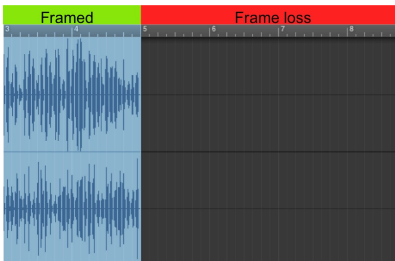
Figure 6 Framing situation in an erroneous ISDN via IP situation, no Reframing due to BONDING
