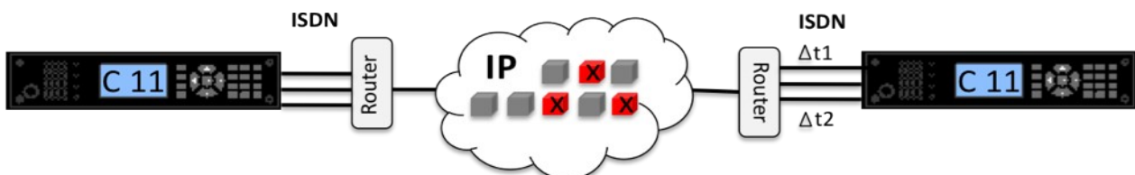
Figure 2 Two C11 Audio Codecs connected via ISDN, but ISDN is routed via IP incl. packet losses
